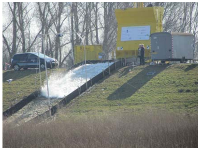
Figure 1: Wave overtopping tests at Nijmegen (top) and Millingen (bottom)
