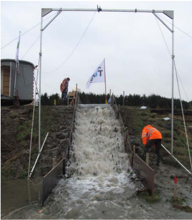
Figure 2: Steady overflow simulation by Flanders Hydraulics Research (MOW)
