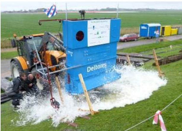
Figure 3 : A wave impact generator in action
